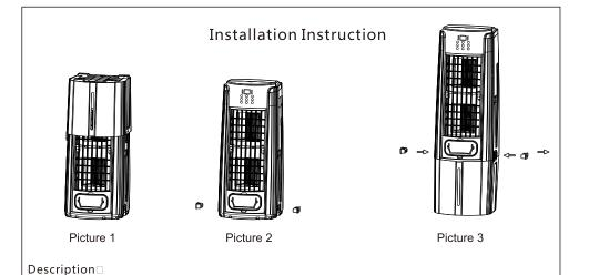
3. Remove the water tank and insert the casters into the bottom hole of the water tank,
